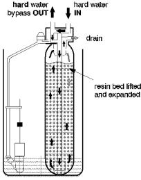
5 FAST RINSE: Backwash is followed by a fast flow of water down through the resin tank. The fast flow packs the resin bed and gets it ready for return to service (FIG. 9).
